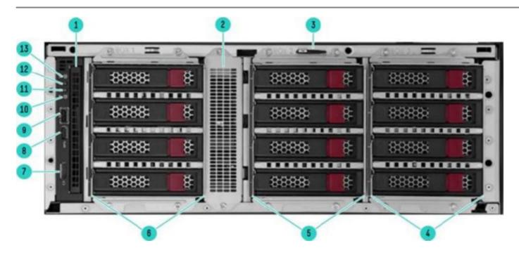
Front View - LFF chassis with optional Gen11 4LFF HDD Cage Kits shown (Rack mode)
